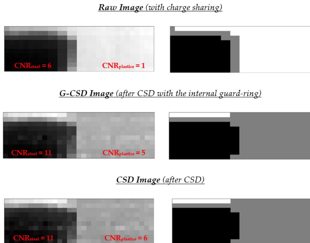
Figure 15. On the left side, the grayscale raw, the G-CSD and the CSD images from the tested phantom, presented in photon counting (PC) mode. On the right side, the results of the material segmentation (k-means clustering): the gray zone for coffee, white for plastics and black for steel. The segmentation is well done after partial (G-CSD) and total rejection (CSD) of the charge sharing events, while a poor segmentation is obtained with the raw image (on the first row of the right-side column). The CNR values are also reported.
