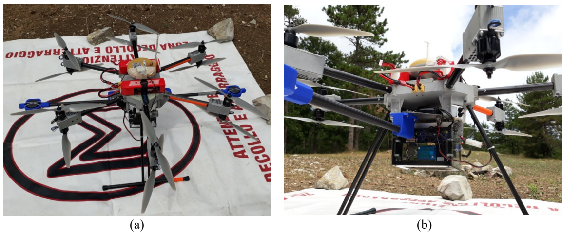
Figure 1. (a) The hexa-coaxial copter; (b) the LasUAV Light Detection and Ranging (LiDAR) system mounted in the unmanned aerial vehicle (UAV).
