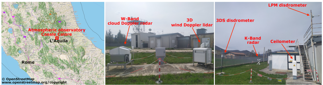
Figure 1. The Casale Calore site with the position of the instruments installed during the CORE-LAQ field campaign.
