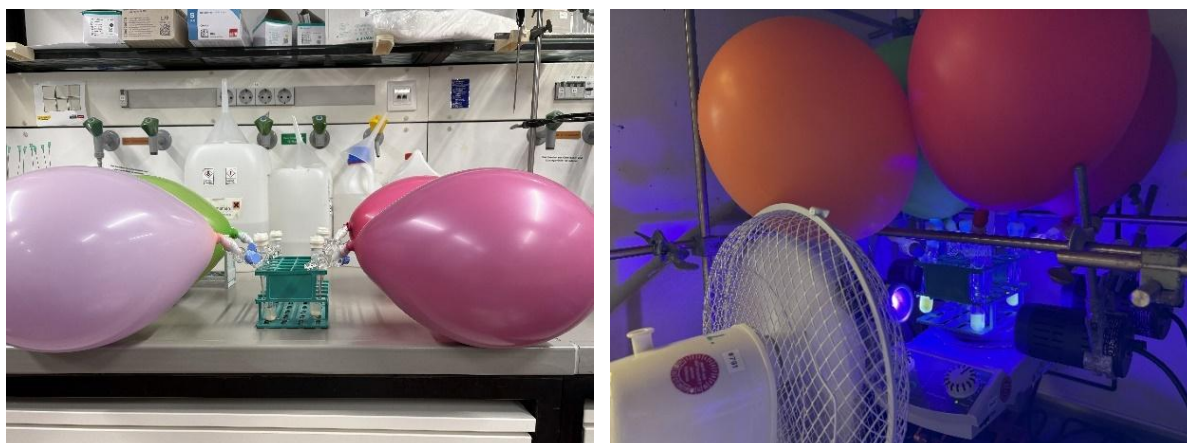
Fig. S4. Set up for the oxidative cleavage of alkenes
