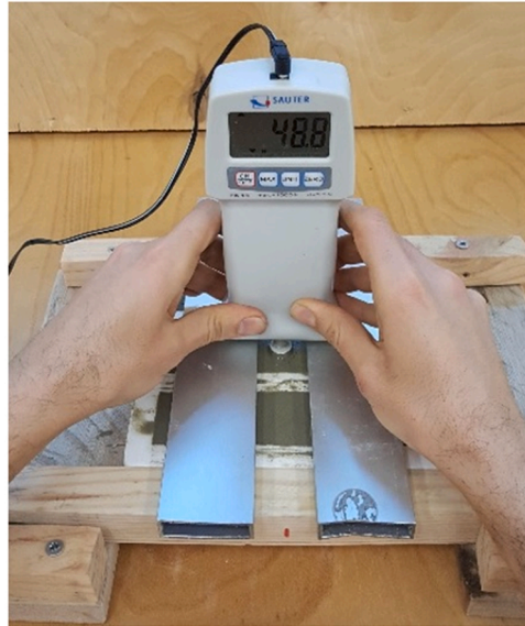
Fig. 6. Penetration phase performed by using the described pocket penetrometer. The depicted mould is made of polystyrene and the displacements are constrained with a wood block device [30].
