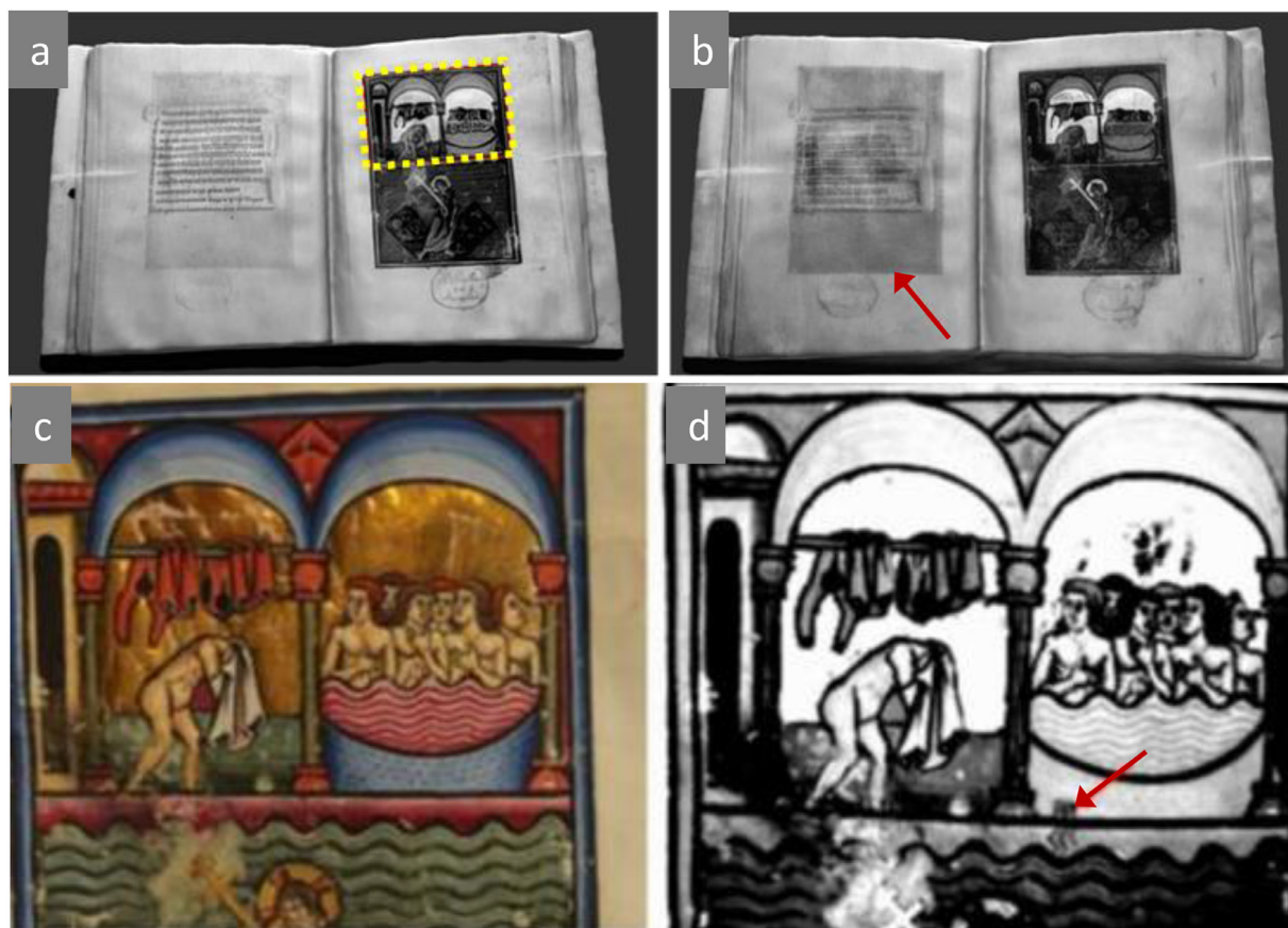
Fig. 8. Carta 9 verso and carta 10 recto, De Balneis Puteolaneis. Model obtained from the thermograms recorded a) soon after the pulse and b) at larger delays. c) Magnification and d) corresponding thermogram of the area marked by the dashed rectangle in Fig. 6a. The arrow in Fig. 6d) indicates a pentimento consisting in a jellyfish.
