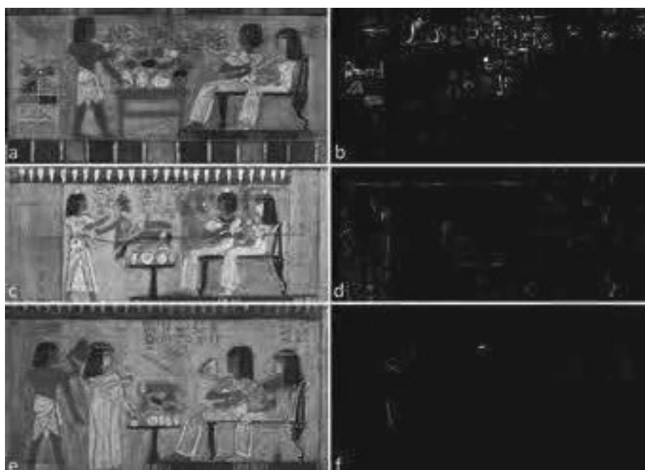
Fig. 4. Comparison of the Visible image of the three caskets (a: S.8212; c: S.8213; e: S.8613) and the corresponding detail (b, d, f) where white areas show the distribution manganese acquired by MA-XRF.
