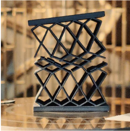
Fig. 6: Origami structure after failure in the austenite phase
