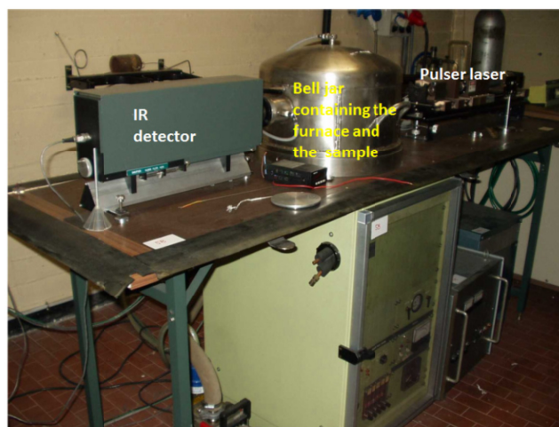
Fig. 4. The experimental layout consists (from right to left) in a laser, a bell jar containing the furnace and the sample holder, and an infrared detector. The data acquisition system is placed on the back side of the apparatus.
