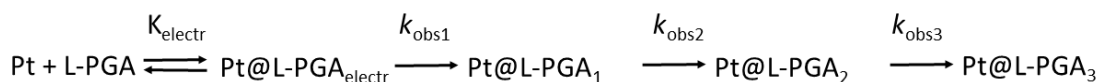
Scheme 2. Proposed mechanistic pathway for the formation of the supramolecular adduct of [Pt(terpy)Me]Cl on L-PGA.
