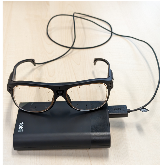
Fig. 1. The Tobii Pro Glasses 3 kit, composed of the wearable glasses unit connected to a portable computing unit that provides storage and connectivity.
