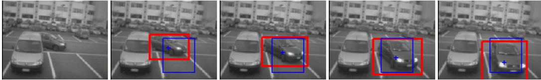
Figure 1.6 Car detection and analysis of parking lot occupancy status.
