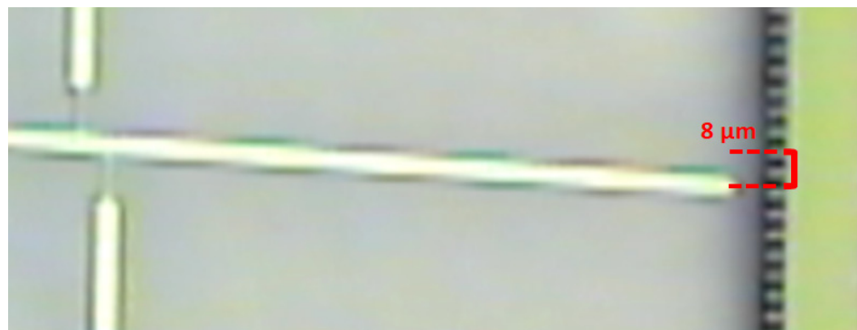
Figure 13. Shift of strain gauge indicating bar (sample P2) after release from the substrate.
