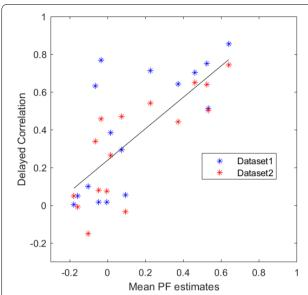
**Fig. 6** Scatter plot showing the relationship between mean PF estimates (horizontal axis) and delayed correlation (vertical axis) on the two sensory-motor experiments. On both results taken altogether the Pearson's correlation coefficient  $\rho$  is 0.74, which corresponds to a statistically significant correlation with p < 0.001. Slope and offset of the linear fit were 0.83 and 0.24 respectively
