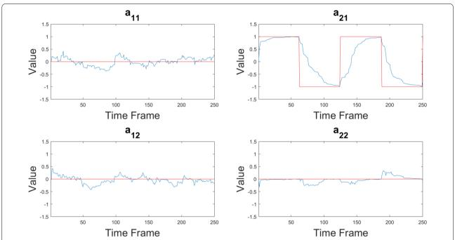
**Fig. 4** Time courses of the hidden parameters  $a_{ij}$  in the case of a 2-node network with non-stationary coefficient  $a_{21}$  alternating between 1 and -1. Red lines represent the true values, while blue lines represent the estimates obtained by PF
