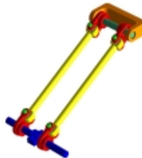
Fig. 7 – A parallelogram module composed by two struts on Fig 1
