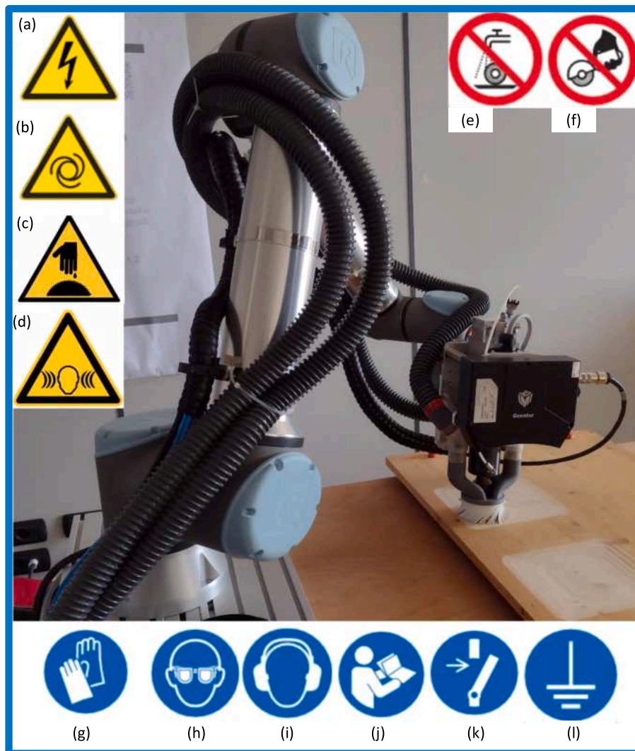
Fig. 25. Safety issues about the ScarfingTool.
