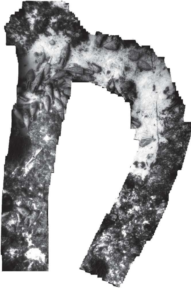
Figure 4: Optical mosaic map. The image results from the stitching process of 61 frames captured by a Basler ACE GigE camera during an experimental campaign performed at the Cala Minnola site, in front of the Levanzo Island, Sicily.
