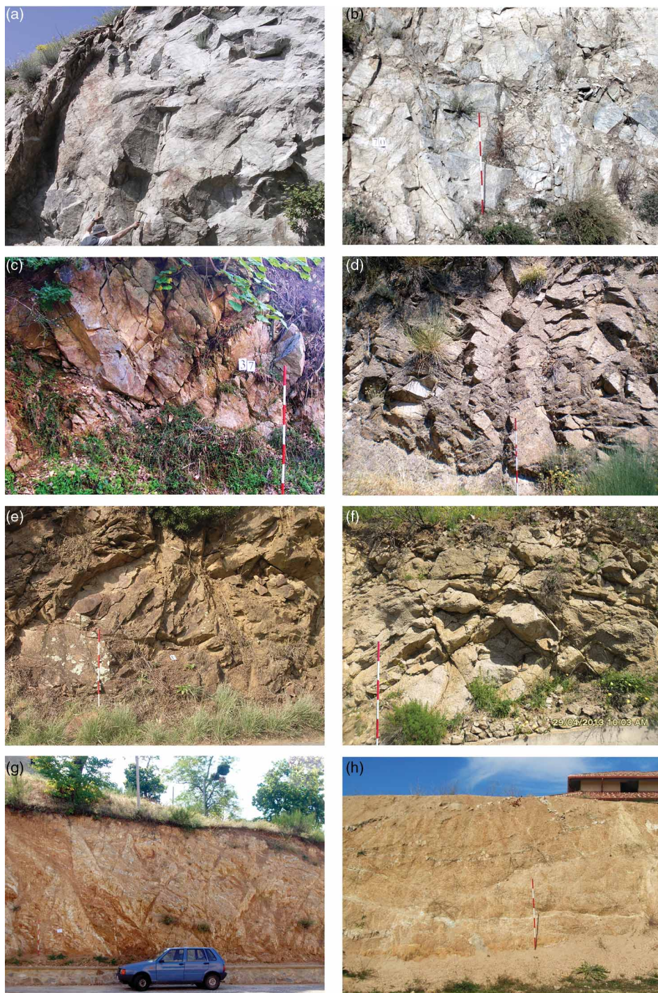
Figure 9. Examples of weathering classes surveyed in the study area and effects of weathering increase upward from slightly weathered rocks (class II) to completely weathered rocks (class V): (a) gneiss class II; (b) granitoid class II; (c) gneiss class III; (d) granitoid class III; (e) gneiss class IV; (f) granitoid class IV; (g) gneiss class V; and (h) granitoid class V.
