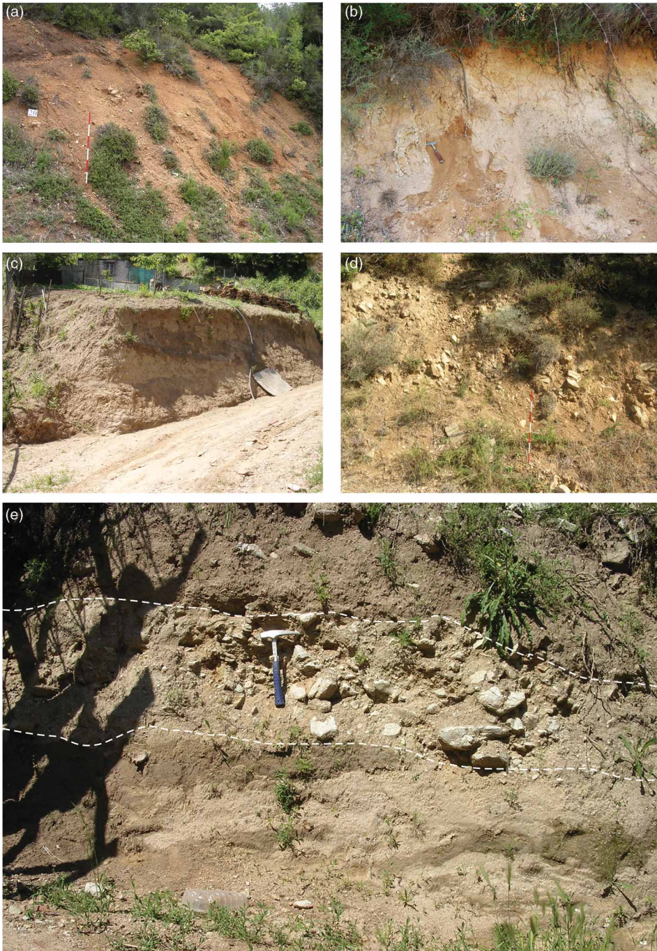
Figure 10. Examples of terrains (in situ weathered soils and transported soils) grouped in class VI: (a) residual soils from gneiss; (b) residual soils from granitoid; (c) colluvial soils; (d) detrital deposits; and (e) alternating colluvial and detrital deposits.
