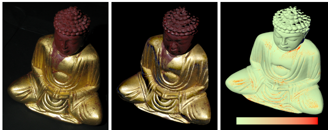
Figure 18: Result using a dataset acquired with the Bonn Dome. We compare a photo (left) that was not used to produce the result using our system (center), and show the color scale difference (right). There is a more significant error around the neck due to a small variation on the rendered shadow.
