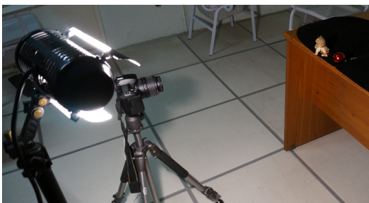
Figure 2: An illustration of the system setup, containing the camera, a light source, a reflective sphere and the object.
