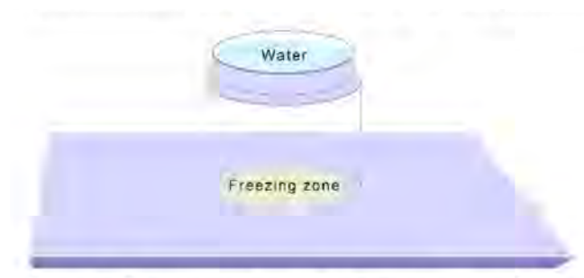
Figure 3. Experimental set up for freeze/thaw test. Water contained in the plastic cylinder was allowed to ice in contact with the surfaces.
