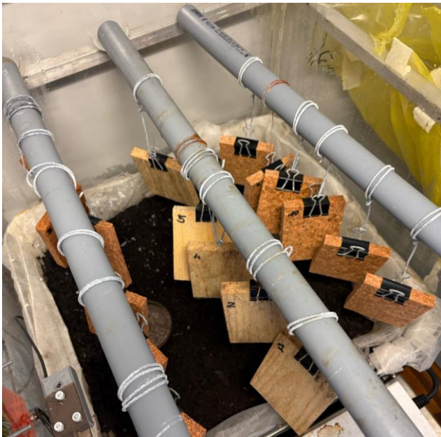
Figure 15 Vsualization of mould test from the top of the box without the pitch roof.
