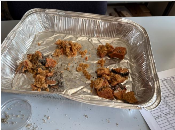
Figure 22 AC PCM specimens at the end of the test, completely destroyed.
