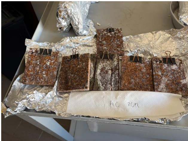
Figure 18 AC with PCM at the end of the test
