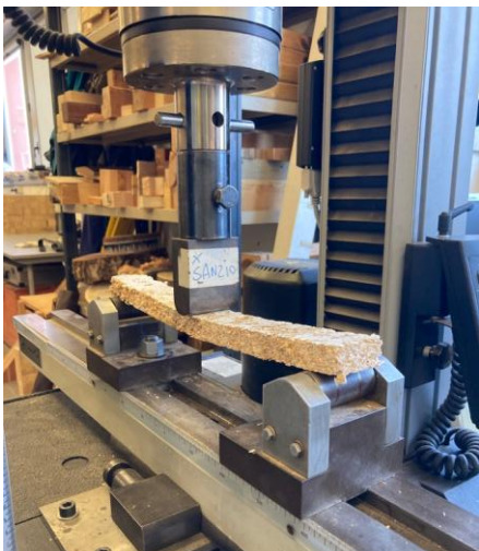
Figure 32 Three points bending test after rupture of sample I_P7
