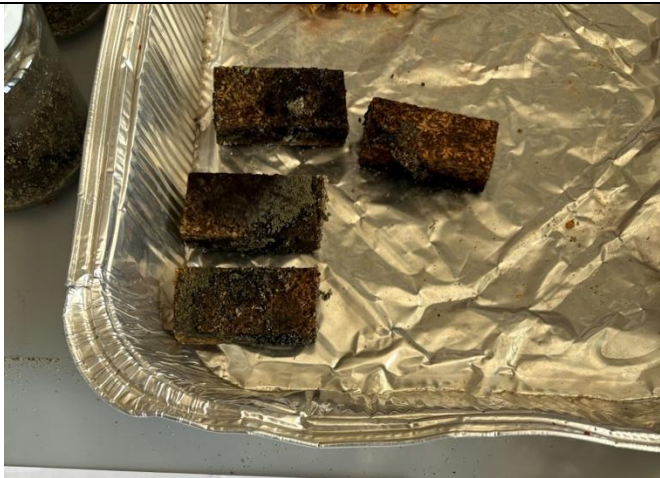
Figure 24 AC no PCM with moulds at the end of the test
