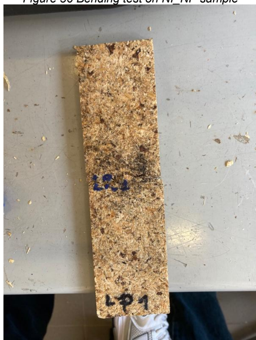
Figure 38 Rupture on lignosulfonate sample a with bio-PCM
