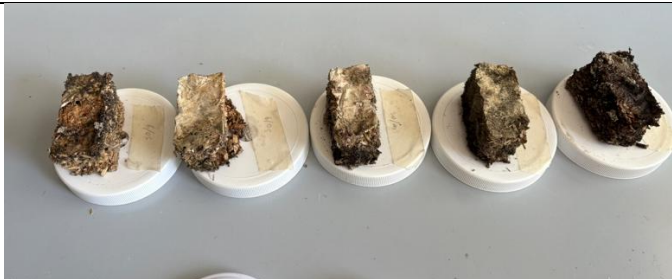
Figure 26 NI_NP mycelium bio-composites at the end of the test. Moulds on the surface
