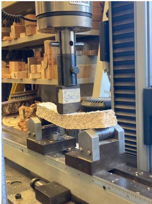
Figure 36 Bending test on NI NP sample
