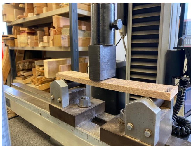
Figure 27 AC-23 specimen, bending test
