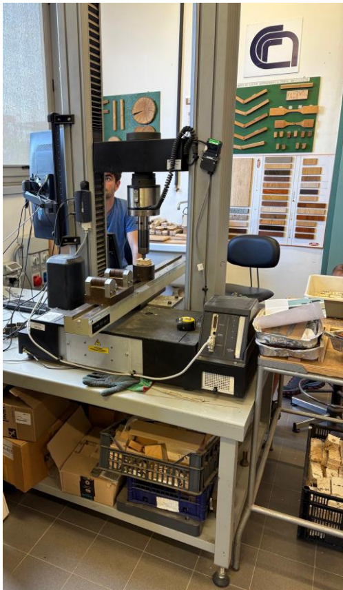
Figure 42 Hardness test on mycelium bio-composites
