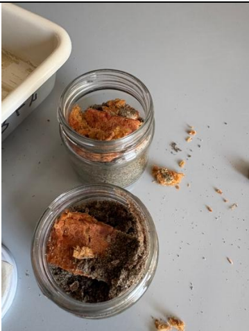
Figure 23 AC PCM completely swollen at the end of the test
