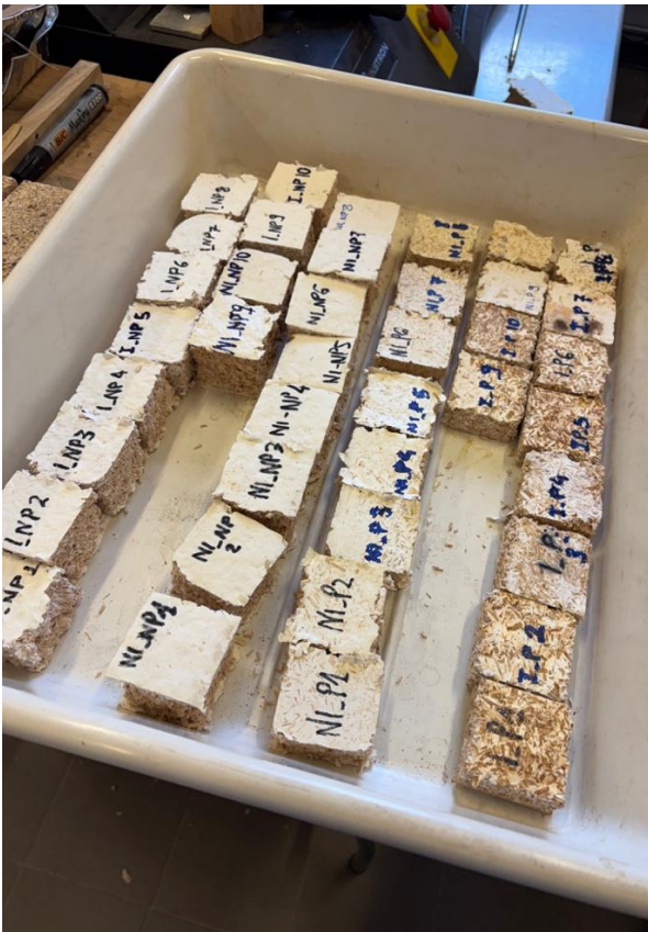
Figure 43 Mycelia specimen after hardness test
