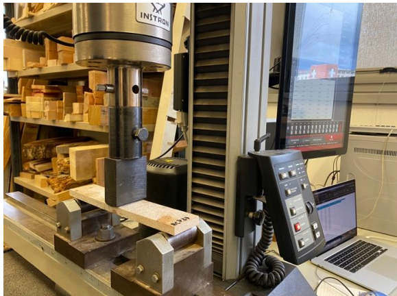
Figure 30 Three points bending test equipment
