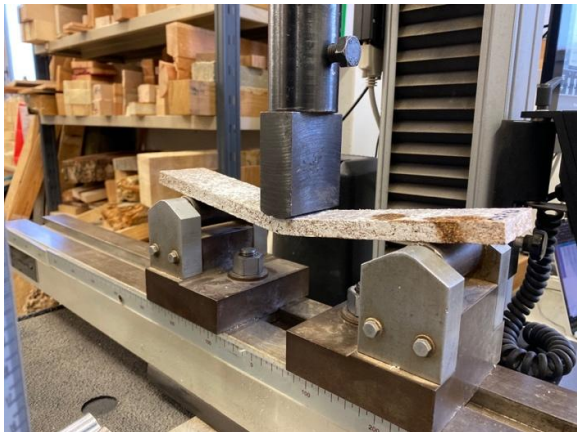
Figure 31 Three points bending test after rupture of sample
