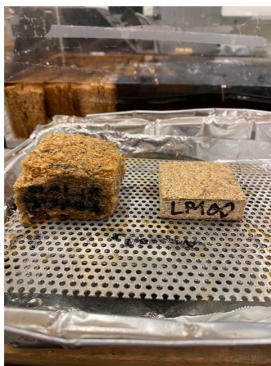
Figure 39 Two specimens with lignosulfonate-based binder compared, before (right) and after (left) the diving
