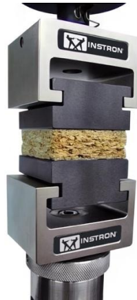
Figure 29 Explanatory figure of the internal bonding test.
