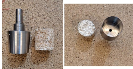
Figure 47 Cutting tool used for the preparation of specimens from mycelia-based boards
