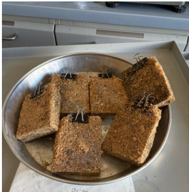
Figure 20 Lignin at the end of the test, the specimens are swollen
