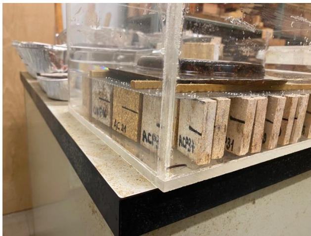
Figure 28 AC, AC-(n)P, OX, OX-(n)P specimens in diving for volumetric swelling test
