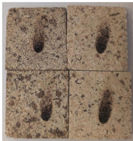
Figure 62 BOKU samples after subjecting to the single flame test. Left: bioPCM containing samples. Right: control samples without bioPCM.
