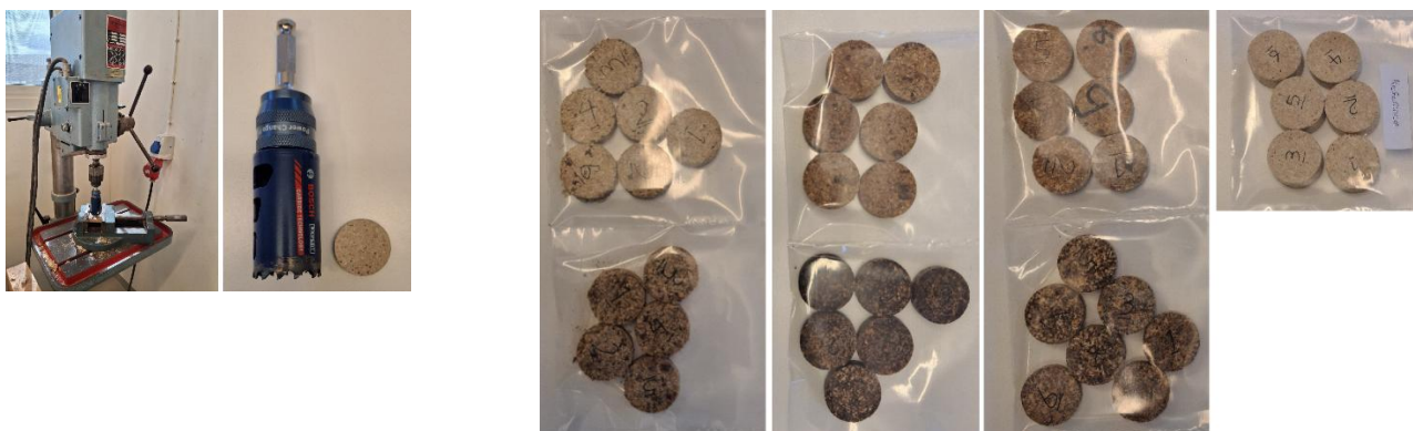
Figure 46 Stationary drilling machine equipped with a circular cutting tool and the circular cutting tool with a representative circular specimen (left); the groups of tested specimens (right)
