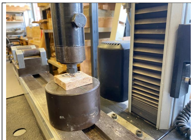
Figure 40 AC-32P Hardness Test Specimen
