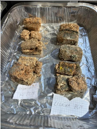
Figure 25 Lignosulfonate bio-composites with PCM, on right, and without PCM at the end of the test
