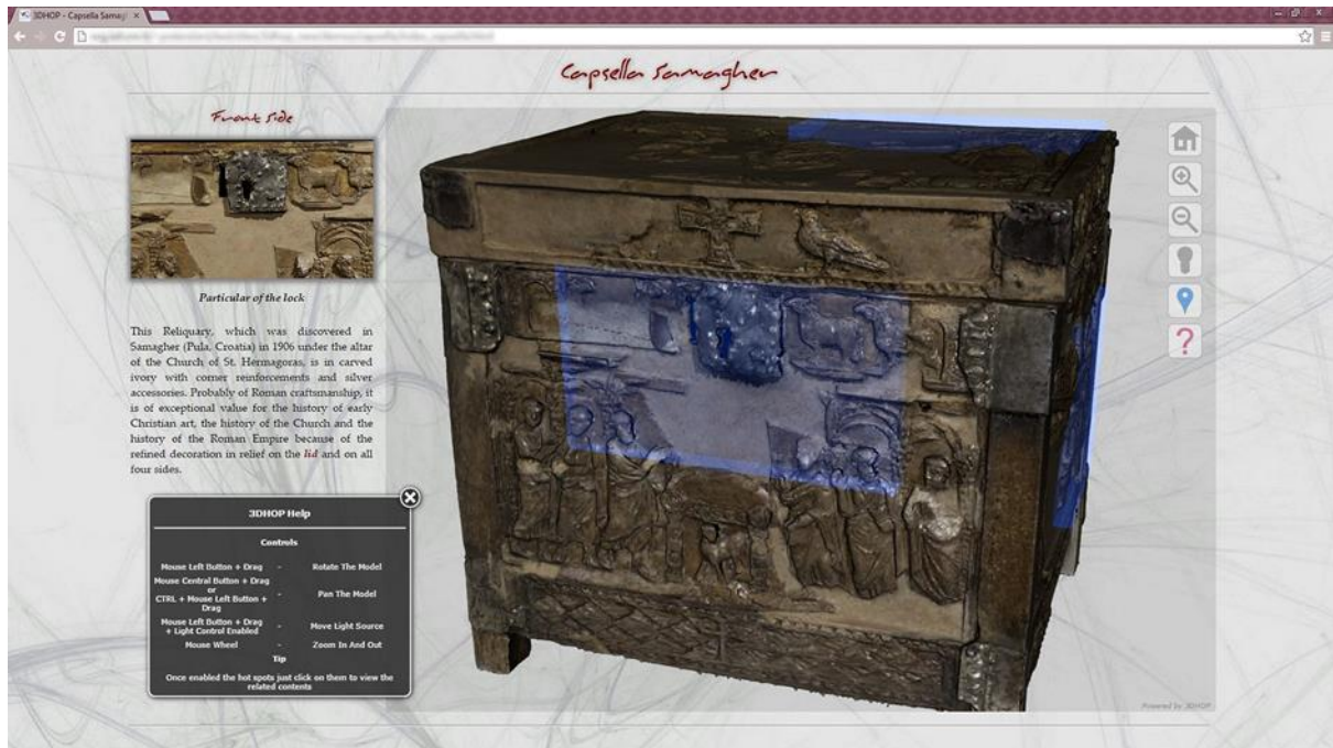
Figure 4: A 3DHOP application developed by CNR-ISTI. In this example, a high-resolution 3D digitization (10 million triangles) of the Capsella Samagher, an antique reliquary, is presented with additional information (images and text). These information are linked to the 3D geometry through geometric hotspots (light-blue regions).
