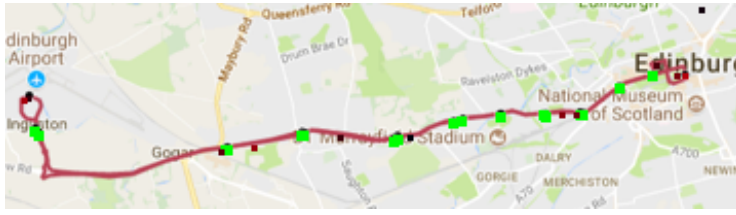
Fig. 13: One state in the generated model. Buses are colour-coded according to their direction, fleet number, and current delay. Bus stops are painted in green.
