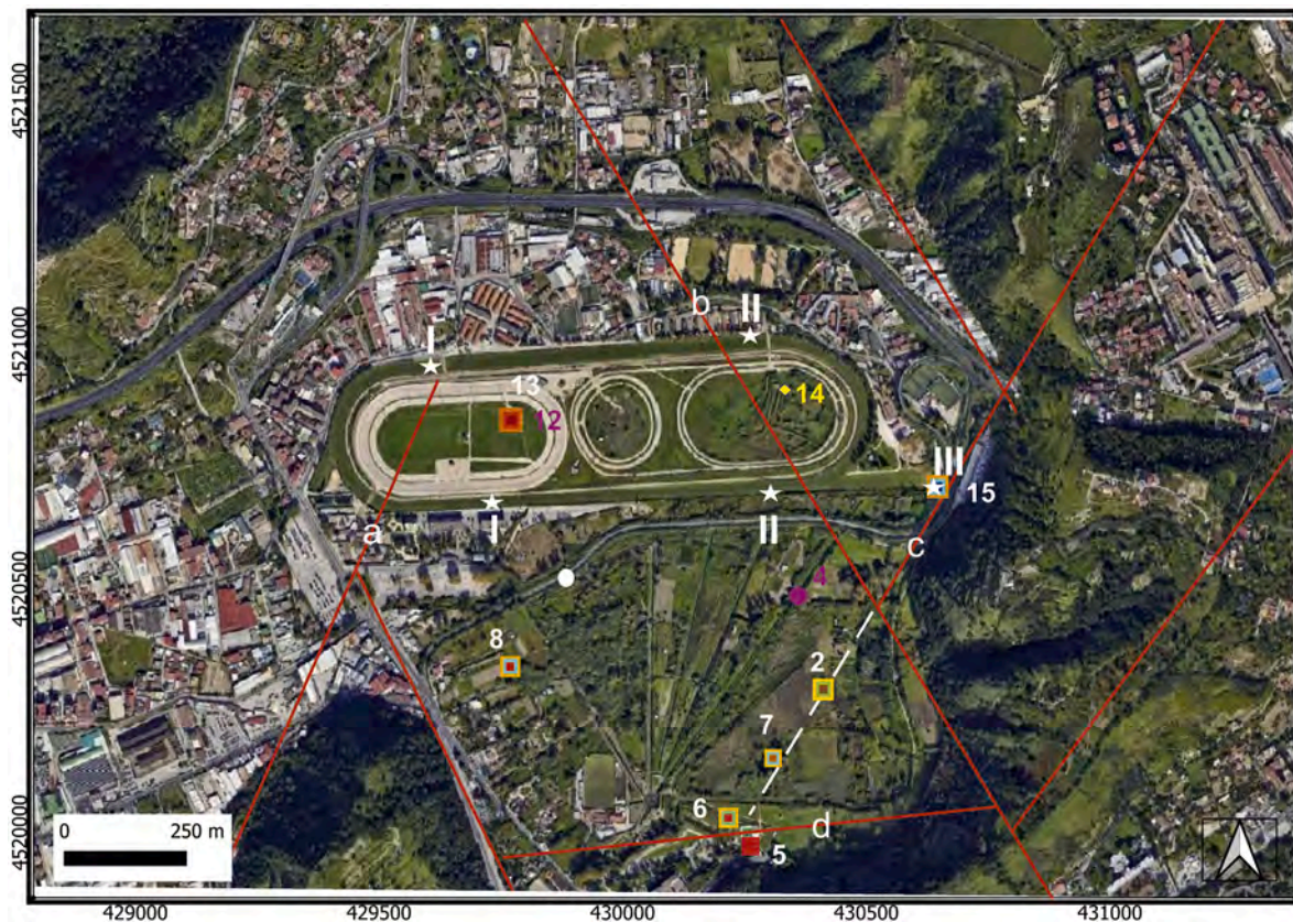
Fig. 15. Orthophoto image (from Google Earth) with superimposition of previously known faults (Red Lines) after Isaia et al., (2015) . White stars and labels for gravimetric anomalies I, II and III for both north and south profile. Squares, circle and numbers for wells sampled for Physico-chemical and stratigraphic analysis meanings as Fig. 12 . White dot hot spring today hidden by highway foundations (Data from Plans for agricultural land Società Napoletana per le Terme di Agnano). White dashed line for alignments of water samples with T > 25.5\text{ }^{\circ}\text{C} , \text{Cond} > 2000\text{ }\mu\text{S/cm} and \text{HCO}_3 values comprise from 600 to 1600 mg/l.
