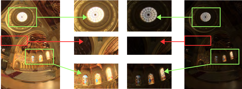
Figure 1: Example of two TMOs that take into account two different aspects. On the left side, the contrast in the bright (green squares) and dark areas (red square) is preserved but the detail in the windows is not well reproduced. On the right side, the detail in the windows is well reproduced (i.e., the global contrast is well reproduced), but the detail in the dark areas are not preserved. The original image is copyright of Paul Debevec.
