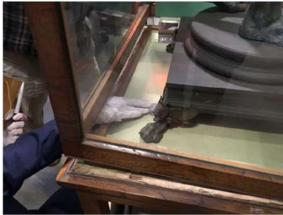
Figure 3 - Insertion of a small node in a show-case of the Egyptian Museum of Cairo for continuous monitoring of temperature and relative humidity
