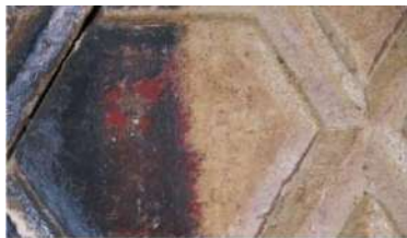
Fig. 15. TEST OF THE STONE BLACK CRUST SANDBLASTING
