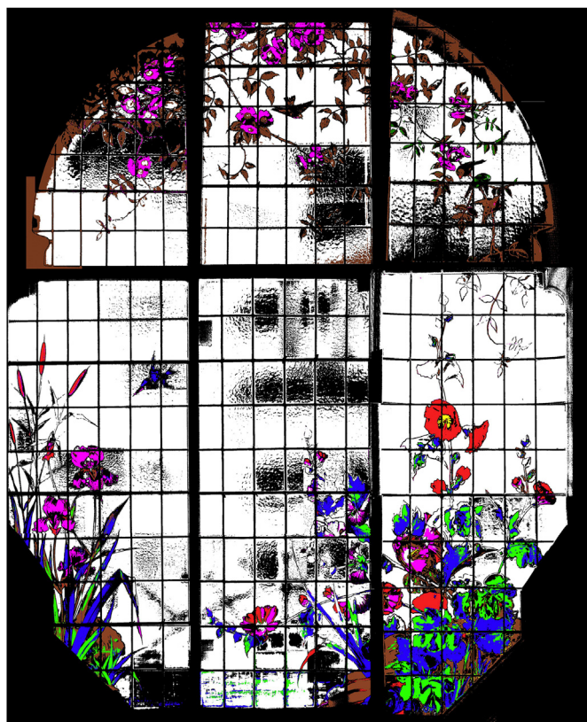
Fig. 7. False-color mapping of the different chromophores in the window panel from the Atelier of the Casa-Museu Dr. Anastácio Gonçalves. Transmittance spectra from each false-color are represented in Fig. 8.
