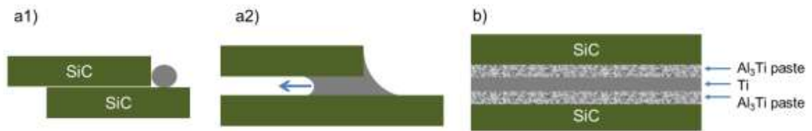
Figure 2: a1) scheme of the capillary infiltration assembly; a2) scheme of the infiltration method mechanism; b) scheme of the Al 3 Ti-Ti-Al 3 Ti paste assembly.
