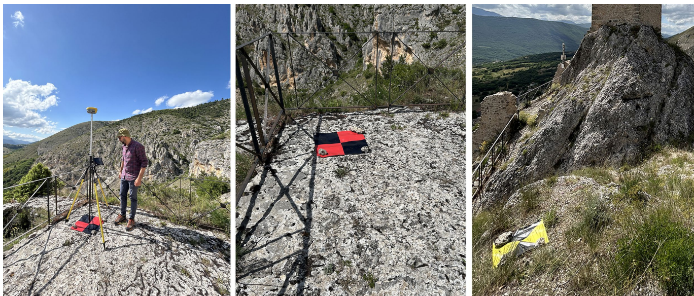
Figure 6. Positioning and measurement of Ground Control Points (GCP).
