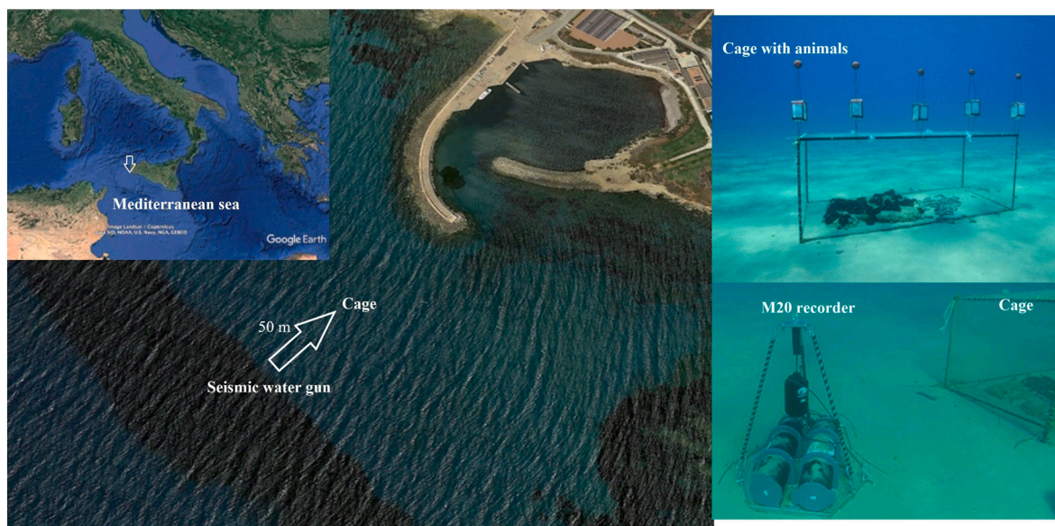
Fig. 1. The position of the cage within sea urchins on the bottom, and M20 recorder. In the insert, the location of Capo Granitola (Sicily Strait, Italy) laboratory was showed.
