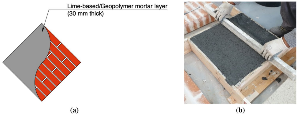
Fig. 6 NHL and GPM samples: a schematic view and b sample preparation
