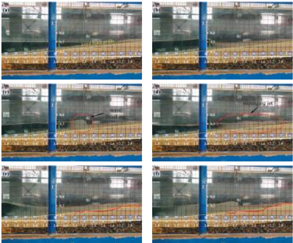
Figure 5. Snapshots (25 fps) of the wave breaking process and the accompanying change in the coral sand beach profile for a water depth of h = 0.3 m, a wave height H = 0.07 m, and wave period of T = 1.8 s. (a) t = 0 s, (b) t = 8.84 s, (c) t = 9.56 s, (d) t = 10.8 s, (e) t = 10 min, (f) t = 30 min. The yellow dashed line is the initial beach profile and the red solid line is the beach profile under wave action.
