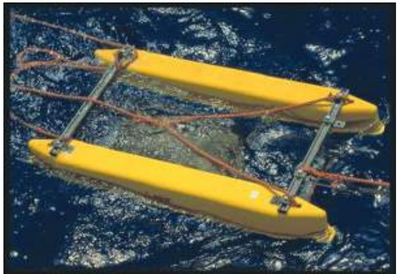
Figure 2. The Uniboom seismic source.
