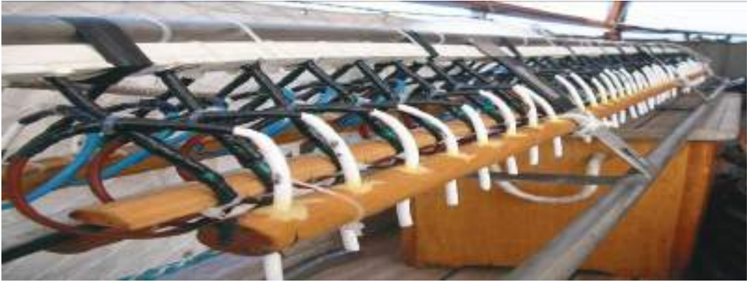
Figure 1. SAM 96: Sparker Array Multi-tip (96 electrodes), developed in the framework of the PNRA (Programma Nazionale Ricerche Antartide) [6].
