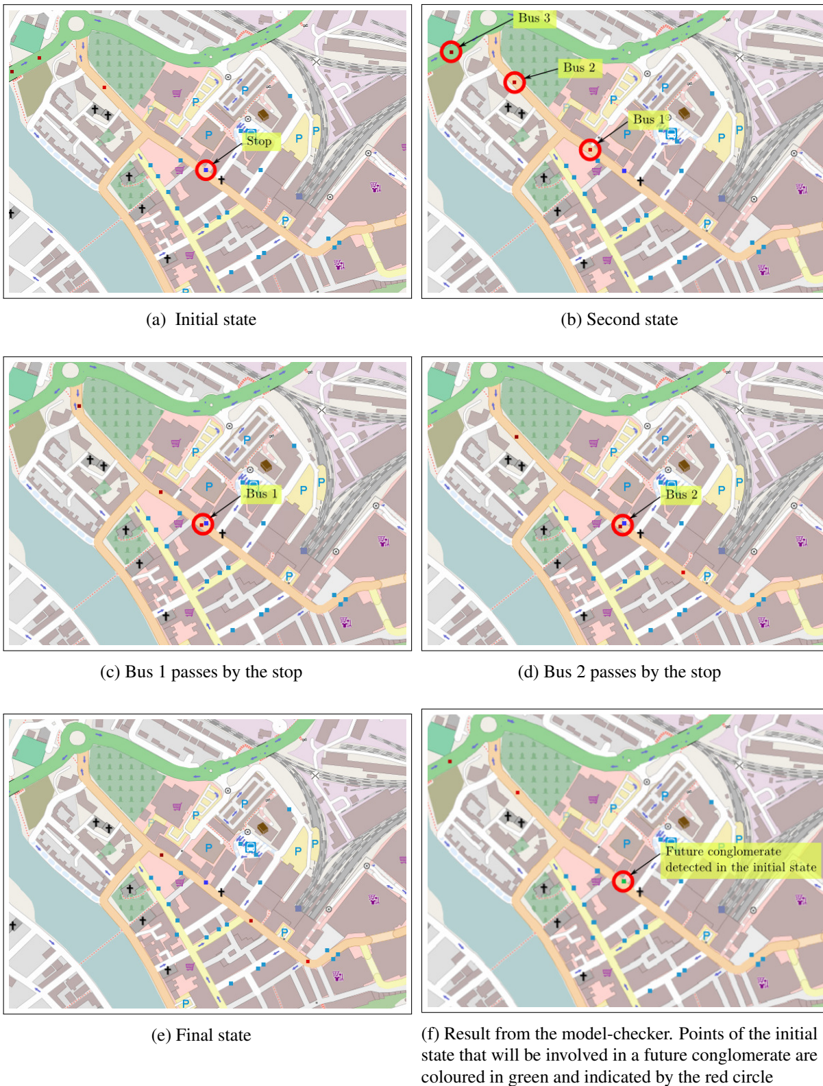
Figure 8: Detection of spatio-temporal conglomerate when bus 1 (c) and bus 2 (d) pass by the same bus stop (a) within a very short time period.
