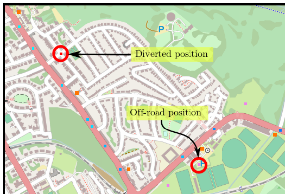
Figure 6: Diverted positions (neither off road, nor on a main street) are automatically highlighted in red by the spatial model checking procedure, off-road positions are highlighted in violet.
