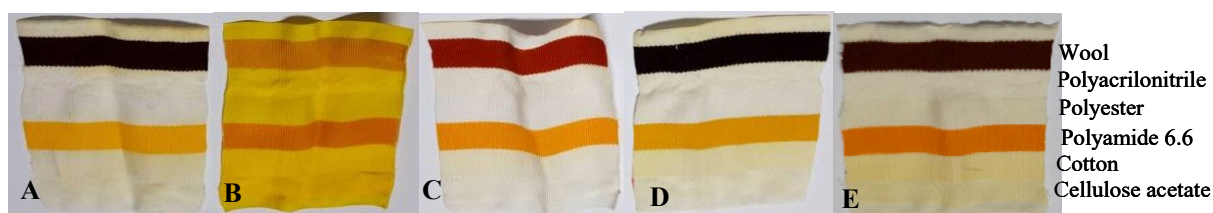
243 Fig. 5 results of the dyeing process on the multifibers textile fabric; A) -Bromocresol purple;
