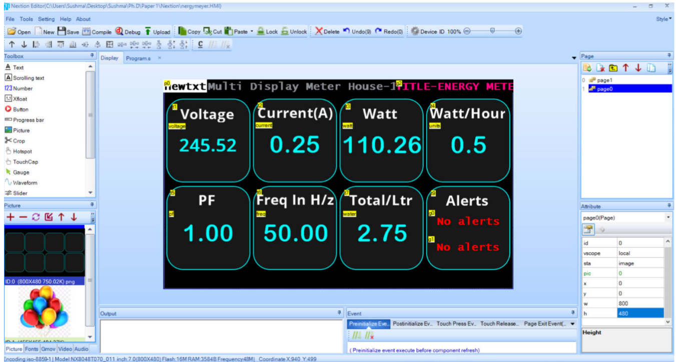
FIGURE 17. GUI designed using nextion editor.
