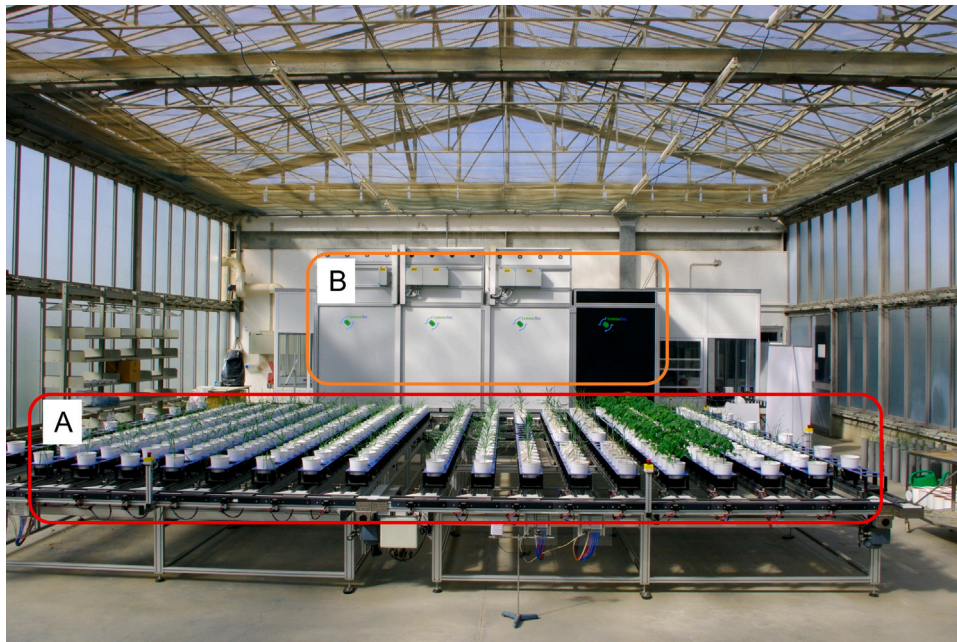
Fig. 1. The setup used for dataset gathering. The foreground of the image (A) contains the plant storage system with conveyor belts that carry the plants to the imaging chambers. The background of the image (B) contains the imaging chambers, which are for, from left to right (the actual direction of plant travel), soil NIR, fluorescence, visible light and plant NIR imaging.
