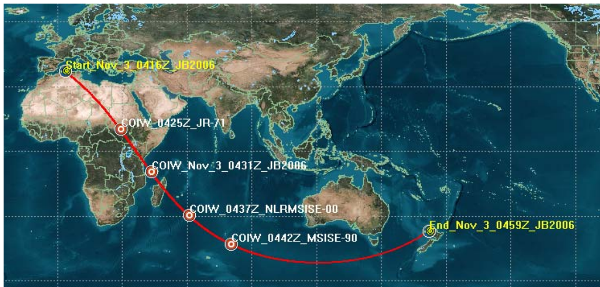
Fig. 14. Last EAS reentry prediction with the TLE of 3 November 2008, 02:14 UTC. The centers of the impact windows (COIW) obtained with the four atmospheric density models are shown, together with the uncertainty window associated to JB2006.
