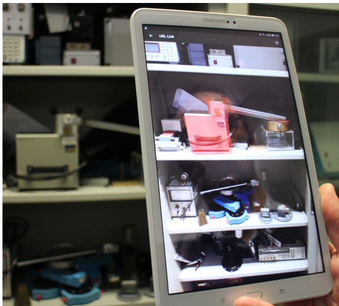
Fig. 4. An example of the use of ARTiCo app in a simulated lab environment, with the item under examination highlighted in AR.
