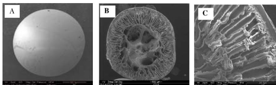
Fig. 4 - SEM pictures of the a) Surface and b,c) Cross-section of the capsules prepared using a film with the pore size of about 500 \mu\text{m} and PEEKWC/DMF 8 wt.%, phase 1, dodecane, phase 2, and water:isopropanol, phase 3.
