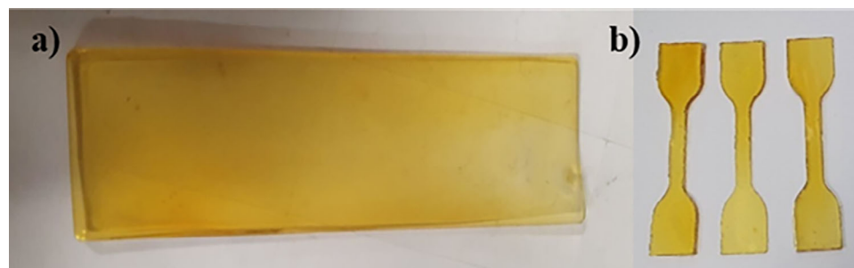
Figure 1. a) Acrylated epoxidized waste cooking oil (AEWCO) cured resin removed from the mould, b) AEWCO dumbbell specimens.
