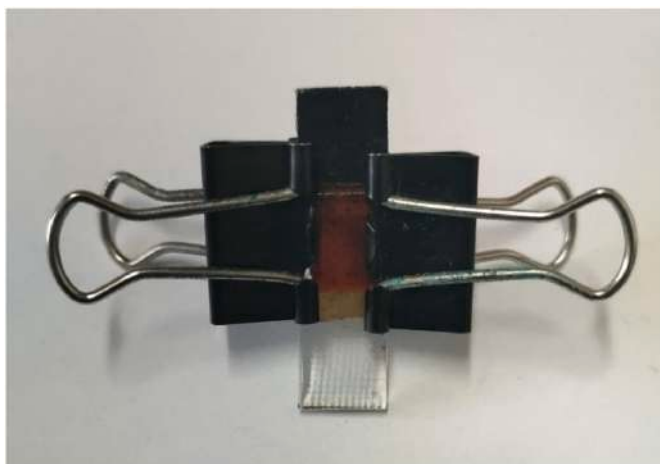
Fig. 2. Picture of the 0.25 cm 2 lab-scale cell with the hematite (orange), the GDL (black) and the two paper clips.
