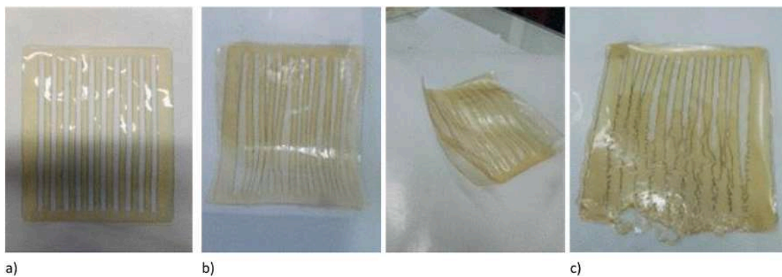
Fig. A.3. 3-layer segmented membrane. (a) The laser-cut flow field, (b) an adhesion test using the hydroalcoholic ionomer. As can be seen from two points of view, the adhesion obtained was not optimal, and the drying process led to the detaching of layers, (c) using an alcoholic ionomer as adhesive, partial solubilization of the membrane occurred.
