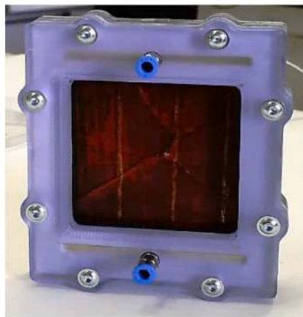
Fig. A.5. Unit cell with broken FTO glass.
