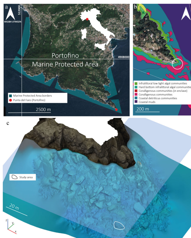
Figure 1. The study site in the Marine Protected Area of Portofino (Punta del Faro, Italy). (a) The border of the Marine Protected Area; (b) a detailed view of the benthic biocenosis mapped in the location of the study site using shapefiles available from [37]; (c) 3D view of the seabed around the study site at Punta del Faro (white polyline) generated via SfM using imagery collected on site.
