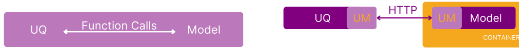
Fig. 3. Monolithic coupling of UQ and model software in a single application (left); UM-Bridge providing a universal interface between UQ and model applications (right). UM-Bridge integrations (“UM”) handle network communication behind the scenes. Optionally, models may be containerized.
