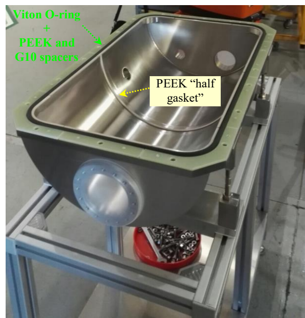
Fig. 6. Mock-up realized to test the VTSS vacuum-tight electrical-insulated crossed joints
