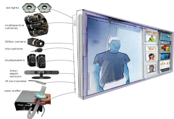
Fig. 1. The Wize Mirror is a multisensory platform which collects videos, images, 3D scans of the human face and gas concentration signals, looking for signs correlated with cardio-metabolic risk.
