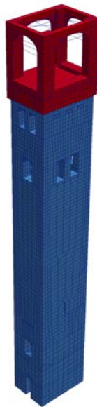
Figure 5: FE mesh of the Clock Tower
