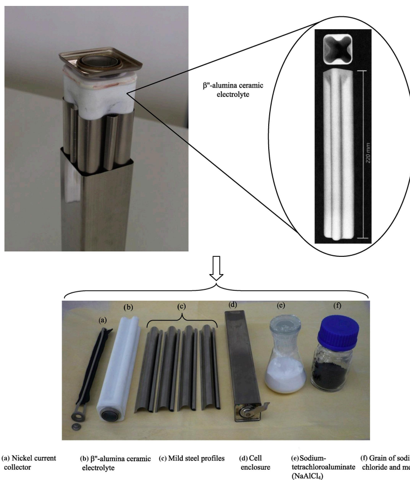
Figure 12. Constructional elements of current commercial Na-NiCl 2 cell. Reprinted from [15], copyright 2015, with permission from Elsevier.
