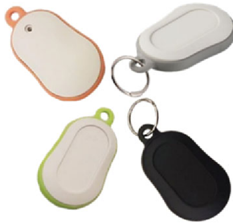
Fig. 4 Social (black) beacons and Environmental (white) beacons: devices suitable to monitor respectively the user social interactions and the user in-house habits during daily life activities. They provide two environmental parameters: house temperature and humidity
