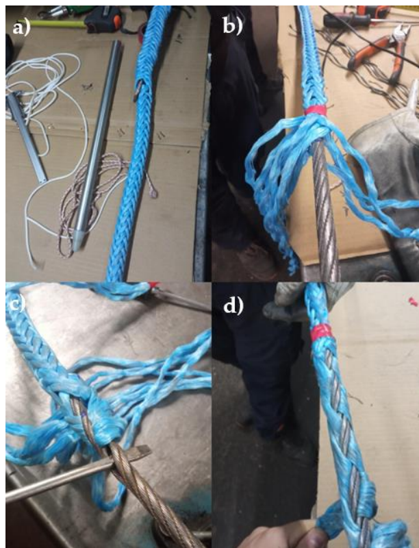
Figure 3. Hybrid splice fabrication process steps: (a) conic steel core introduced with support of purpose-made needle (b) unbraiding up to the conic steel core is supported by a loop of tape (red) to avoid accidental unbraiding; (c) loose synthetic strands are joined in three bunches and braided intercalated under two consecutive steel strands and; (d) final layout of the braided hybrid splice.
