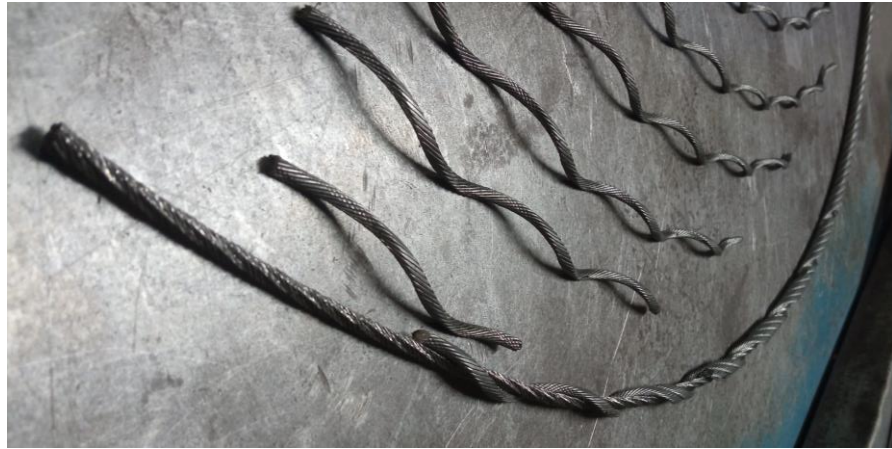
Figure 2. The final layout of the conic steel core is visible in the bottom and on the right side. Above it, strand sections of different lengths are aligned.
