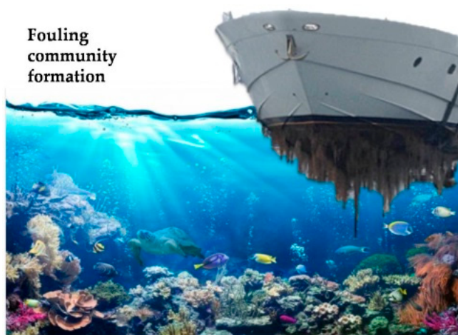
Figure 8. Illustration of the undesirable accumulation of marine biofouling on artificial surface immersed in seawater.
