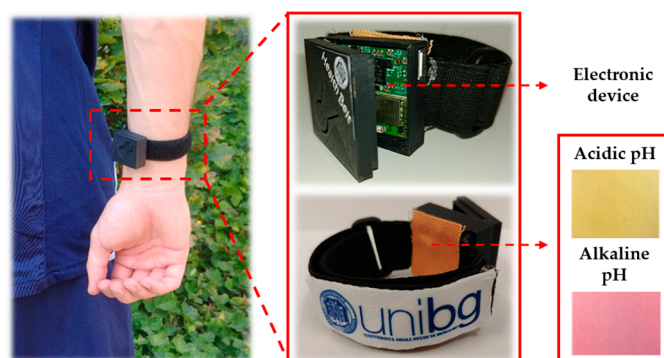
Figure 4. Prototype “Health Belt” for the real-time monitoring of sweat pH.
